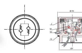
f = Air Filter V1 = Safety Valve V2 = Suction Valve G = NBR seal
